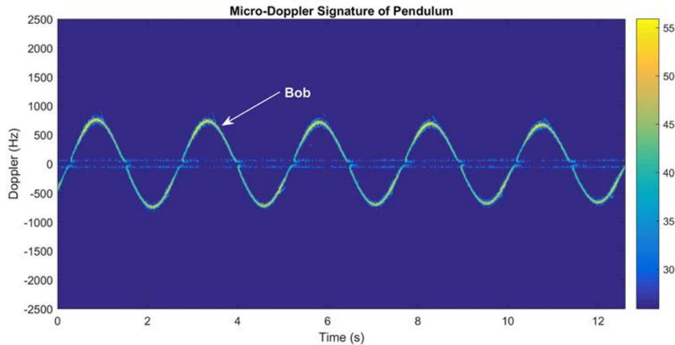
Fig. 4. Experimental result shows micro-Doppler signature of an oscillating pendulum.
