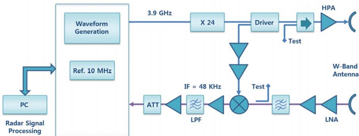
Fig. 3. Block diagram of 94 GHz Doppler radar system.
