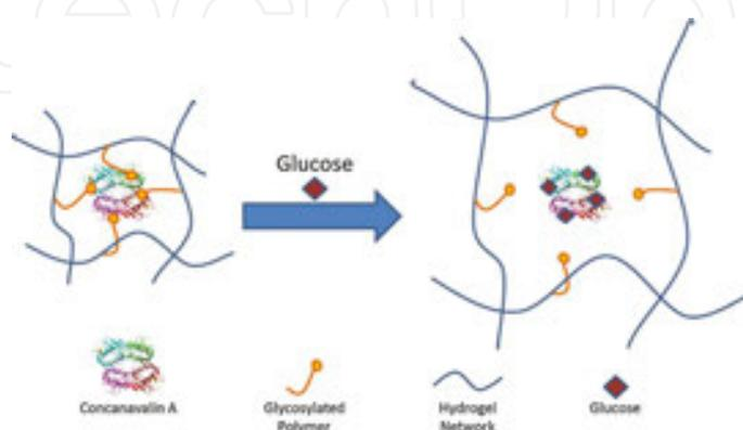
**Figure 19.** Concanavalin A-based glucose-responsive hydrogel swelling mechanism.
