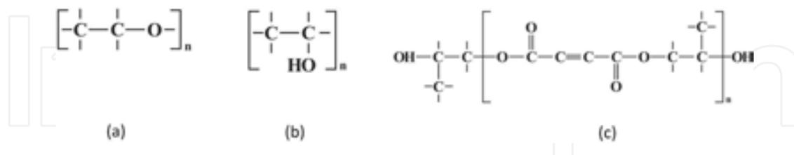
**Figure 15.** Structure of synthetic hydrogel-forming polymers: (a) PEO, (b) PVA (100% hydrolyzed), and (c) PPF.
