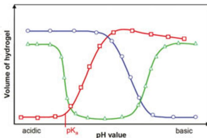
**Figure 11.** Phase transition behavior of polyelectrolyte hydrogels. Acidic hydrogels ( $\square$ ) are ionized by deprotonation in basic solutions. Basic hydrogels ( $\circ$ ) swell in acidic solutions due to the ionization of their basic groups by protonation. Amphiphilic hydrogels ( $\Delta$ ) contain both acidic and basic groups, therefore they show two-phase transitions.
