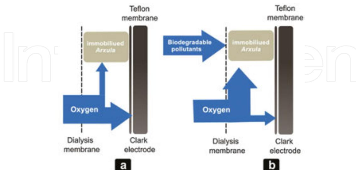
**Figure 20.** Schematic diagram of the *A. adenivorans* LS3 microbial sensor illustrates the microbial consumption of dissolved oxygen (a) before and (b) after the addition of biodegradable pollutant.
